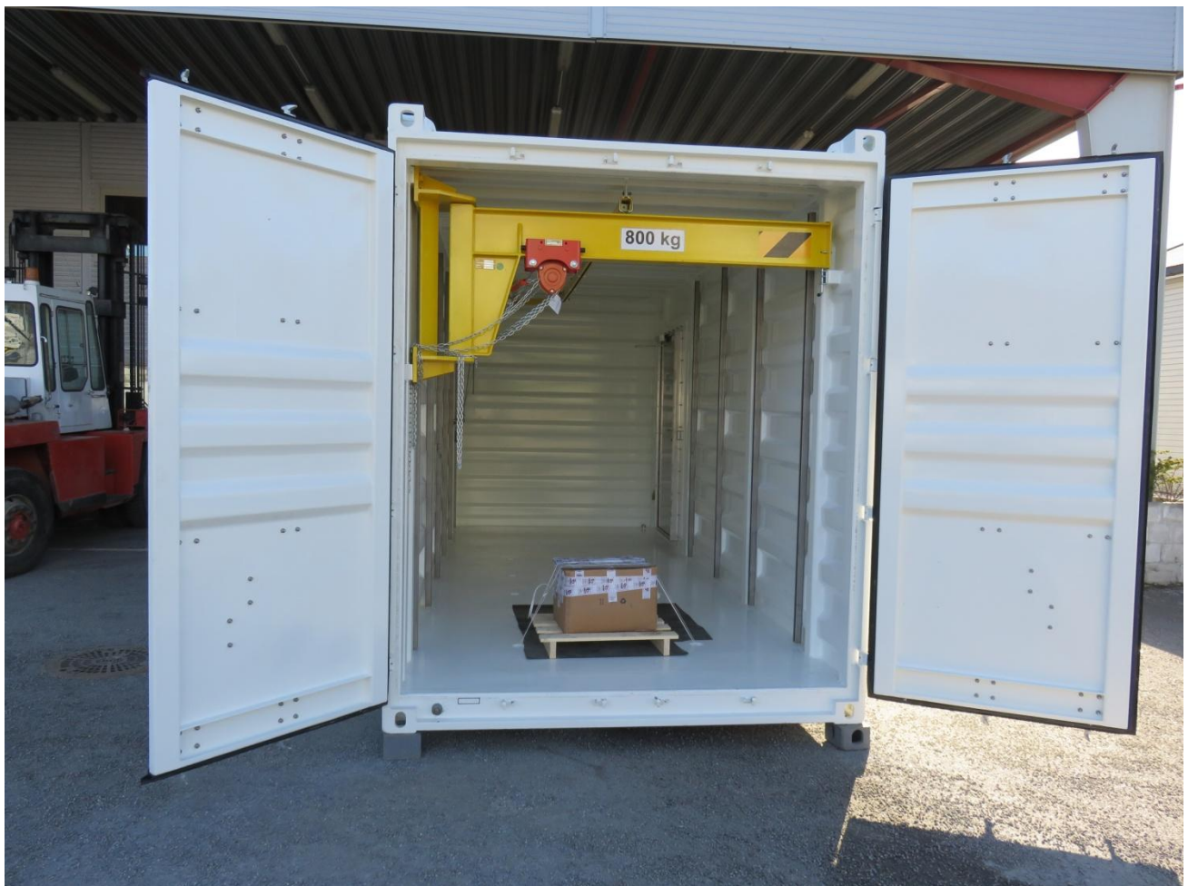
Internal view of the container, showing the opened container gates, swing crane, unistruts etc.
